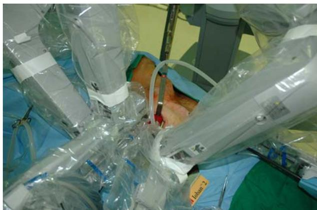
**Fig. 1** The robotic operation. Four robotic arms were placed through the patient's axilla and anterior chest wall trocar
