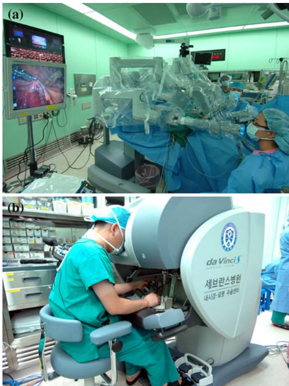
FIG. 1 Operation theater with the da Vinci® Surgical System (a) and an operator at the master console (b)
